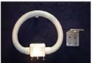
Commercial grade Outdoor Matched Loop Antenna, supplied with HD L-Mount bracket, can be used with RG-59 or RG-6Quad Cable up to 30m long. Ideal for building applications and easy to use DIP Switch configuration for Installers. (Freq. range 520 to 1725KHz)
