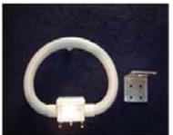
Heavy duty weather proof construction, Narrowband Fixed Frequency AM Loop with BNC connector, L-Mounting Bracket. Either 75 Ohms standard, 50 Ohms, or F-Female connector available on request.
