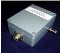
1:1 Coaxial choke balun, LF and HF models are available, rated @2KW PEP Gold centre pinned Teflon Insulated SO-239 socket, 6mm Stainless Steel Terminals, S/S Nuts & washers, fitted with S/S Top Mounting Eyelet
